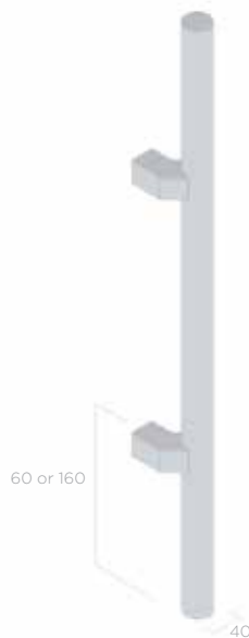
40 diam arcadia rail with TYPE D stanchion
