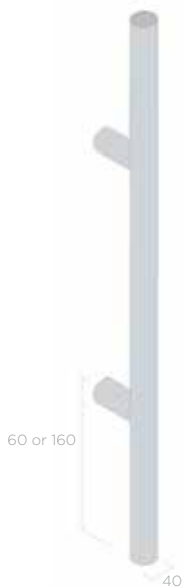
40 diam arcadia rail with TYPE A stanchion
