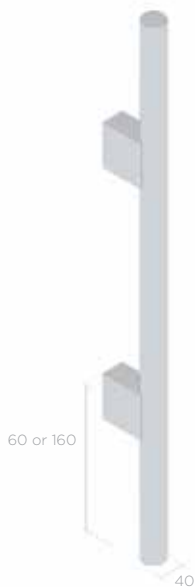
40 diam arcadia rail with TYPE B stanchion
